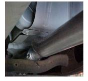
Install head pipe # A onto you're existing stock flange re-using the factory hardware. Use a jack stand to support the converter. Do not tighten. Insert welded hanger into rubber grommet.
