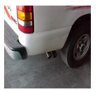
Install the stainless tips. Clamp down. To clean your stainless tips use any stainless cleaner or a Scotch Brite pad. Now go back and tighten all clamps, nuts and bolts. Start from the front and work back.
